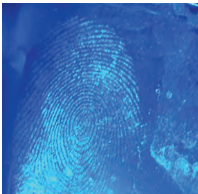
Fig. 2: Blood print developed and enhanced on glass exposed to 5000C using formulation A exposed to 4000C using formulation B
